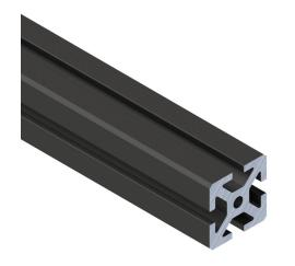
SureFrame 40 Series standard T-slotted rail, black, 6063-T6 anodized aluminum alloy, cut to length, 40 x 40mm profile, slot size 8.
