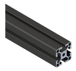
SureFrame 40 Series light T-slotted rail, black, 6063-T6 anodized aluminum alloy, cut to length, 40 x 40mm profile, slot size 8.
