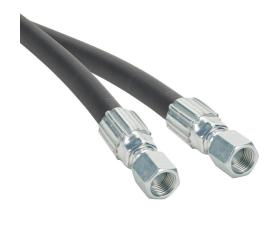
Gates ProFlex petroleum based hydraulic fluid hose assembly, synthetic rubber, braided steel wire reinforced, black, 3/8in inside diameter, 0.65in outside diameter, (2) -6 female straight JIC 37 deg fittings, 8ft working length.
