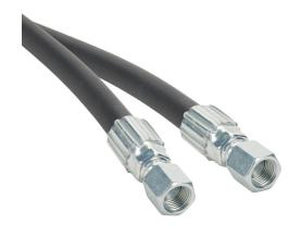
Gates ProFlex petroleum based hydraulic fluid hose assembly, synthetic rubber, braided steel wire reinforced, black, 3/8in inside diameter, 0.65in outside diameter, (2) -6 female straight JIC 37 deg fittings, 6ft working length.
