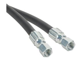
Gates ProFlex petroleum based hydraulic fluid hose assembly, synthetic rubber, braided steel wire reinforced, black, 3/8in inside diameter, 0.65in outside diameter, (2) -6 female straight JIC 37 deg fittings, 2ft working length.
