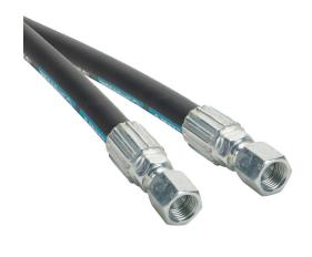
Gates MXT petroleum based hydraulic fluid hose assembly, synthetic rubber, braided steel wire reinforced, black, 3/8in inside diameter, 0.675in outside diameter, (2) -6 female straight JIC 37 deg fittings, 6ft working length.
