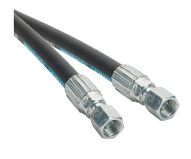
Gates MXT petroleum based hydraulic fluid hose assembly, synthetic rubber, braided steel wire reinforced, black, 3/8in inside diameter, 0.675in outside diameter, (2) -6 female straight JIC 37 deg fittings, 4ft working length.
