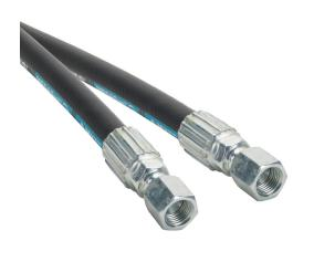
Gates MXT petroleum based hydraulic fluid hose assembly, synthetic rubber, braided steel wire reinforced, black, 3/8in inside diameter, 0.675in outside diameter, (2) -6 female straight JIC 37 deg fittings, 10ft working length.
