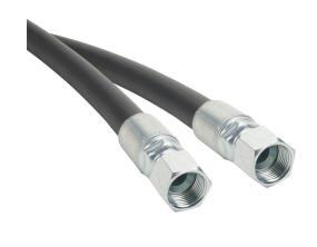
Gates ProFlex petroleum based hydraulic fluid hose assembly, synthetic rubber, braided steel wire reinforced, black, 3/4in inside diameter, 1.08in outside diameter, (2) -12 female straight JIC 37 deg fittings, 6ft working length.
