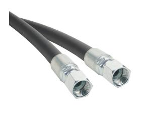
Gates ProFlex petroleum based hydraulic fluid hose assembly, synthetic rubber, braided steel wire reinforced, black, 3/4in inside diameter, 1.08in outside diameter, (2) -12 female straight JIC 37 deg fittings, 2ft working length.
