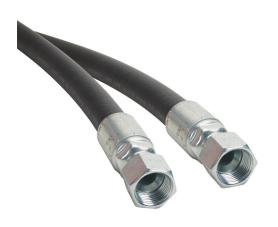
Gates MXT petroleum based hydraulic fluid hose assembly, synthetic rubber, braided steel wire reinforced, black, 3/4in inside diameter, 1.08in outside diameter, (2) -12 female straight JIC 37 deg fittings, 8ft working length.
