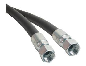
Gates MXT petroleum based hydraulic fluid hose assembly, synthetic rubber, braided steel wire reinforced, black, 3/4in inside diameter, 1.08in outside diameter, (2) -12 female straight JIC 37 deg fittings, 6ft working length.
