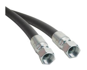
Gates MXT petroleum based hydraulic fluid hose assembly, synthetic rubber, braided steel wire reinforced, black, 3/4in inside diameter, 1.08in outside diameter, (2) -12 female straight JIC 37 deg fittings, 4ft working length.
