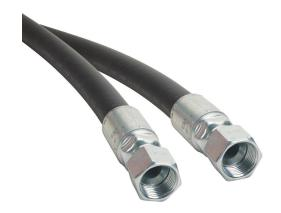
Gates MXT petroleum based hydraulic fluid hose assembly, synthetic rubber, braided steel wire reinforced, black, 3/4in inside diameter, 1.08in outside diameter, (2) -12 female straight JIC 37 deg fittings, 2ft working length.
