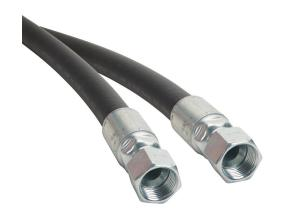
Gates MXT petroleum based hydraulic fluid hose assembly, synthetic rubber, braided steel wire reinforced, black, 3/4in inside diameter, 1.08in outside diameter, (2) -12 female straight JIC 37 deg fittings, 10ft working length.
