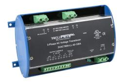
AcuAMP AC voltage transducer, 3-phase, 0-600 VAC line-to-line sensing range, True RMS, (4) 4-20 mA and (1) relay, SPST-N.O. output, 0.5A @ 125 VAC, 1A @ 30 VDC output rating, phase loss @ 360 VAC non-adjustable trip point, 120 VAC operating voltage.
