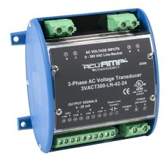
AcuAMP AC voltage transducer, 3-phase, 0-300 VAC line-to-neutral sensing range, True RMS, (4) 4-20 mA and (1) relay, SPST-N.O. output, 0.5A @ 125 VAC, 1A @ 30 VDC output rating, phase loss @ 180 VAC non-adjustable trip point, 24 VAC/VDC operating voltage.
