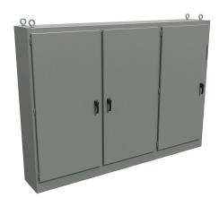
Hammond disconnect enclosure, NEMA 12, right flange, 84 x 119 x 18in (HxWxD), freestanding, carbon steel, ANSI 61 gray, powder coat finish, 3-door, 3-point padlocking handle.
