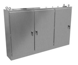
Hammond disconnect enclosure, NEMA 3R/4/4X/12/13, right flange, 72 x 119 x 18in (HxWxD), freestanding, 304 stainless steel, #4 brush finish, 3-door, 3-point padlocking handle.
