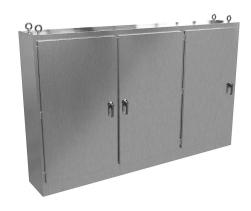
Hammond disconnect enclosure, NEMA 3R/4/4X/12/13, right flange,  $72 \times 119 \times 18$  in (HxWxD), freestanding, 304 stainless steel, #4 brush finish, 3-door, 3-point padlocking handle.
