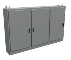
Hammond disconnect enclosure, NEMA 12, right flange, 72 x 119 x 18in (HxWxD), freestanding, carbon steel, ANSI 61 gray, powder coat finish, 3-door, 3-point padlocking handle.
