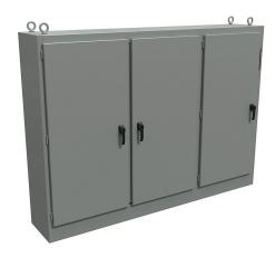
Hammond disconnect enclosure, NEMA 12, right flange, 72 x 101 x 18in (HxWxD), freestanding, carbon steel, ANSI 61 gray, powder coat finish, 3-door, 3-point padlocking handle.
