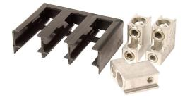
Eaton box type wiring lug, replacement, line or load mount, 2 openings, 400 MCM-500 MCM wire(s). Package of 3. For use with AutomationDirect (Eaton) 600A frame MCCBs. (1) 3-pole terminal cover included.
