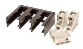
Eaton box type wiring lug, replacement, line or load mount, 2 openings, 400 MCM-500 MCM wire(s). Package of 3. For use with AutomationDirect (Eaton) 600A frame MCCBs. (1) 3-pole terminal cover included.
