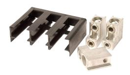
Eaton box type wiring lug, replacement, line or load mount, 2 openings, 2/0-250 MCM or 2/0-500 MCM wire(s). Package of 3. For use with AutomationDirect (Eaton) 400A frame MCCBs. (1) 3-pole terminal cover included.
