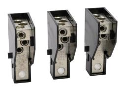
Eaton multi-wire box type wiring lug, load side mount, 225A, 3 openings, #14-2 AWG copper only. Package of 3. For use with AutomationDirect (Eaton) 225A frame MCCBs. Mounting hardware and insulators included.
