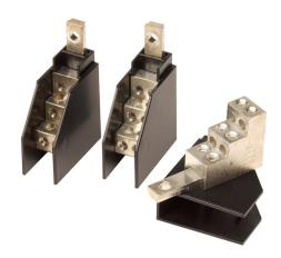
Eaton multi-wire box type wiring lug, load mount, 100A, 6 openings, #14-6 AWG copper only. Package of 3. For use with AutomationDirect (Eaton) 100A frame MCCBs. Mounting hardware and insulators included.
