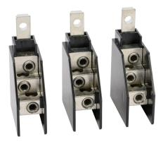
Eaton multi-wire box type wiring lug, load side mount, 100A, 3 openings, #14-2 AWG copper only. Package of 3. For use with AutomationDirect (Eaton) 100A frame MCCBs. Mounting hardware and insulators included.
