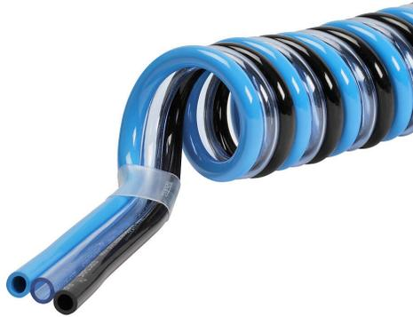
NITRA pneumatic bonded coiled tubing, ether-based polyurethane, black, clear blue and blue, triple 5/32in outside diameter, 0.093in inside diameter, 20 coils, 4.4ft (1.34m) working length.
