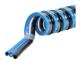
NITRA pneumatic bonded coiled tubing, ether-based polyurethane, black, clear blue and blue, triple 5/32in outside diameter, 0.093in inside diameter, 10 coils, 2.5ft (0.76m) working length.
