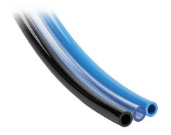
NITRA pneumatic bonded tubing, ether-based polyurethane, black, clear blue and blue, triple 5/32in outside diameter, 0.093in inside diameter, 50ft package.
