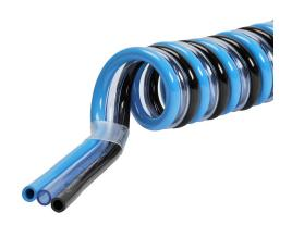
NITRA pneumatic bonded coiled tubing, ether-based polyurethane, black, clear blue and blue, triple 1/4in outside diameter, 0.156in inside diameter, 40 coils, 11.9ft (3.63m) working length.
