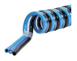
NITRA pneumatic bonded coiled tubing, ether-based polyurethane, black, clear blue and blue, triple 1/4in outside diameter, 0.156in inside diameter, 20 coils, 6.3ft (1.92m) working length.
