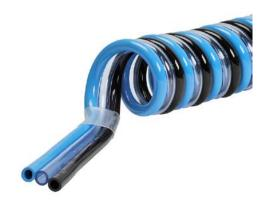
NITRA pneumatic bonded coiled tubing, ether-based polyurethane, black, clear blue and blue, triple 1/4in outside diameter, 0.156in inside diameter, 10 coils, 3.4ft (1.04m) working length.
