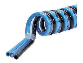
NITRA pneumatic coiled tubing, ether-based polyurethane, black, clear blue and blue, triple 6mm outside diameter, 5/32in (4mm) inside diameter, 20 coils, 6.2ft (1.90m) working length.
