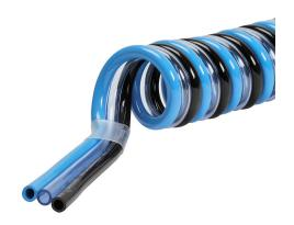
NITRA pneumatic coiled tubing, ether-based polyurethane, black, clear blue and blue, triple 6mm outside diameter, 5/32in (4mm) inside diameter, 10 coils, 3.1ft (0.93m) working length.
