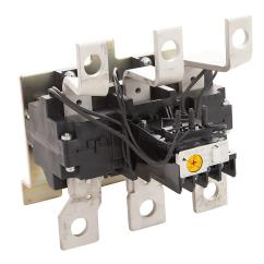
Fuji Electric thermal overload relay, 240.0-360.0A adjustable, bimetallic, direct mount power connection(s), panel mount. For use with 3NC5Hx contactors.
