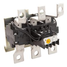
Fuji Electric 3NK5 series thermal overload relay, 200.0-300.0A adjustable, bi-metallic, direct mount power connection(s), panel mount. For use with 3NC5Fx and 3NC5Hx contactors.
