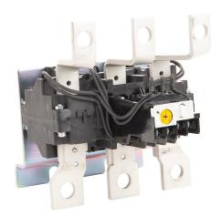
Fuji Electric 3NK5 series thermal overload relay, 160.0-240.0A adjustable, bi-metallic, direct mount power connection(s), panel mount. For use with 3NC5Fx and 3NC5Hx contactors.
