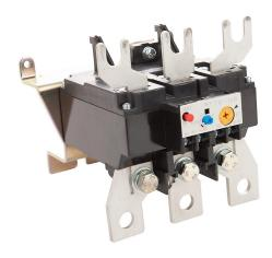
Fuji Electric 3NK4 series thermal overload relay, 125.0-185.0A adjustable, bi-metallic, direct mount power connection(s), panel mount. For use with 3NC4Qx contactors.
