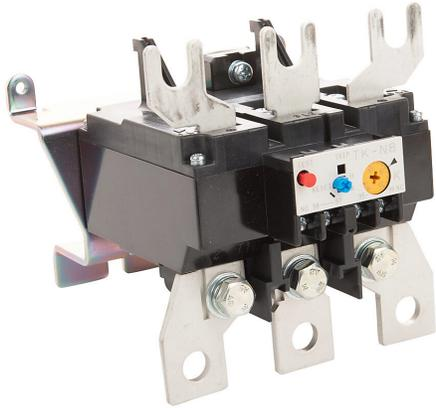
Fuji Electric 3NK4 series thermal overload relay, 85.0-125.0A adjustable, bi-metallic, direct mount power connection(s), panel mount. For use with 3NC4Qx contactors.
