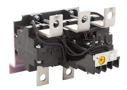
Fuji Electric 3NK4 series thermal overload relay, 160.0-240.0A adjustable, bi-metallic, direct mount power connection(s), panel mount. For use with 3NC4Hx contactors.
