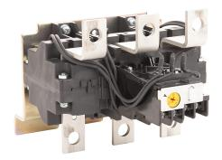
Fuji Electric 3NK4 series thermal overload relay, 125.0-185.0A adjustable, bi-metallic, direct mount power connection(s), panel mount. For use with 3NC4Hx contactors.
