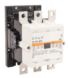
Fuji Electric 3NC5 series IEC contactor, 361A, (3) N.O. power poles, (2) N.O./(2) N.C. auxiliary contacts, 575 VAC (60Hz)/460 VAC (50Hz) coil voltage, low consumption electronic.
