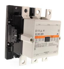
Fuji Electric 3NC5 series IEC contactor, 361A, (3) N.O. power poles, (2) N.O./(2) N.C. auxiliary contacts, 120 VAC (60Hz)/110 VAC (50Hz) coil voltage, low consumption electronic.
