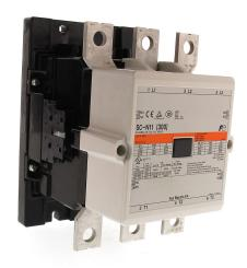
Fuji Electric 3NC5 series IEC contactor, 285A, (3) N.O. power poles, (2) N.O./(2) N.C. auxiliary contacts, 24 VAC/VDC coil voltage, low consumption electronic.
