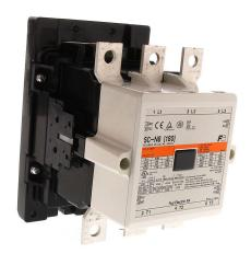
Fuji Electric 3NC4 series IEC contactor, 180A, (3) N.O. power poles, (2) N.O./(2) N.C. auxiliary contacts, 240 VAC (60Hz)/220 VAC (50Hz) coil voltage, low consumption electronic.
