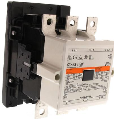
Fuji Electric 3NC4 series IEC contactor, 180A, (3) N.O. power poles, (2) N.O./ (2) N.C. auxiliary contacts, 240 VAC (60Hz)/220 VAC (50Hz) coil voltage, low consumption electronic.
