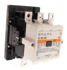
Fuji Electric 3NC4 series IEC contactor, 180A, (3) N.O. power poles, (2) N.O./(2) N.C. auxiliary contacts, 120 VAC (60Hz)/110 VAC (50Hz) coil voltage, low consumption electronic.
