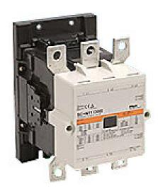
Fuji Electric 3NC4 series IEC contactor, 221A, (3) N.O. power poles, (2) N.O./(2) N.C. auxiliary contacts, 24 VAC/VDC coil voltage, low consumption electronic.
