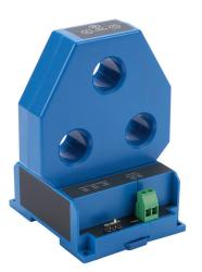
AcuAMP AC current transducer, 3-phase, fixed core, 0-30, 0-50, or 0-100A selectable sensing range, True RMS, 4-20 mA output.
