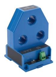
AcuAMP AC current transducer, 3-phase, fixed core, 0-10, 0-15, or 0-30A selectable sensing range, True RMS, 4-20 mA output.
