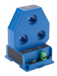
AcuAMP AC current transducer, 3-phase, fixed core, 0-10, 0-15, or 0-30A selectable sensing range, 4-20 mA output.
